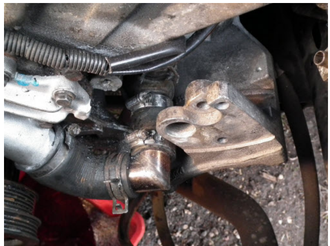
8. AC pump bracket goes back on - bottom pivot first
