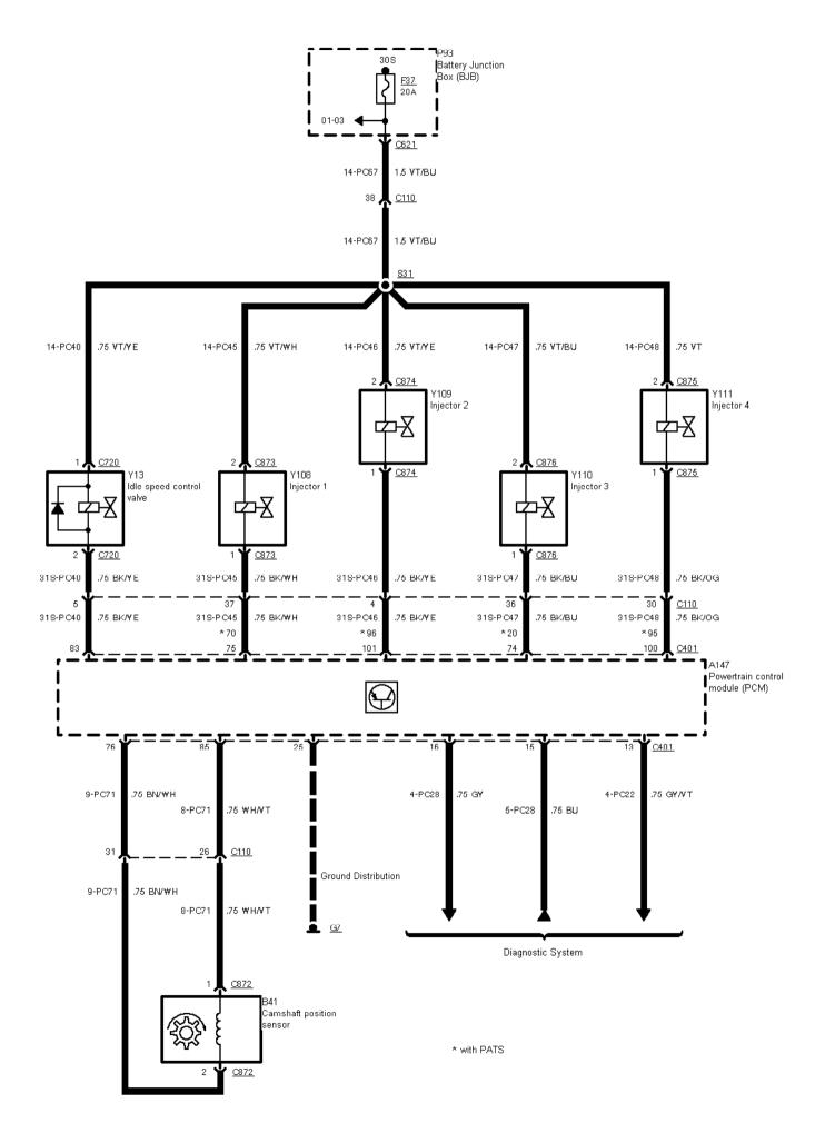
29-02-006 , Engine Control 2,0 I 8V/16V EFI (Manual Transmission) , 2,0 I 8V EFI from 02/95 to 03/96 and as of 04/97
